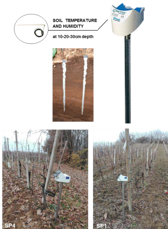
Figure 4: Soil sensors installed in Demo farms, top part sensors scheme, bottom part some example of sensors installed in the vineyards
